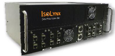
The receivers are linked by one shielded Ethernet cable back to a central command location and connected to an IsoLynx decoder. This is connected to a computer. If robotic cameras are being used, each camera is connected to the command position by two cables; one for camera tracking commands, and one for video download.
